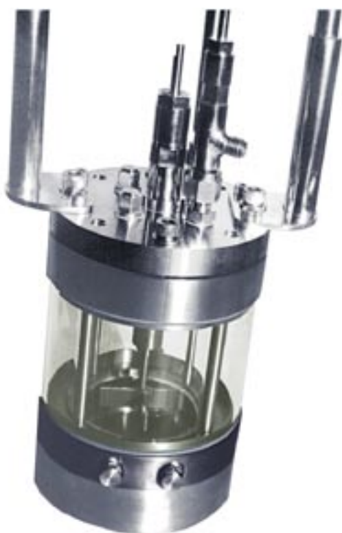
Tantalum reactor for pressures up to 20 bars.
