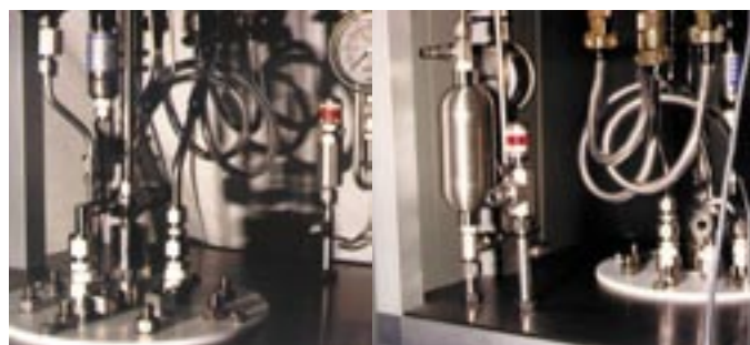
Reactor lid installed in the bench unit. Pressurised shaft seal with armature shown.
