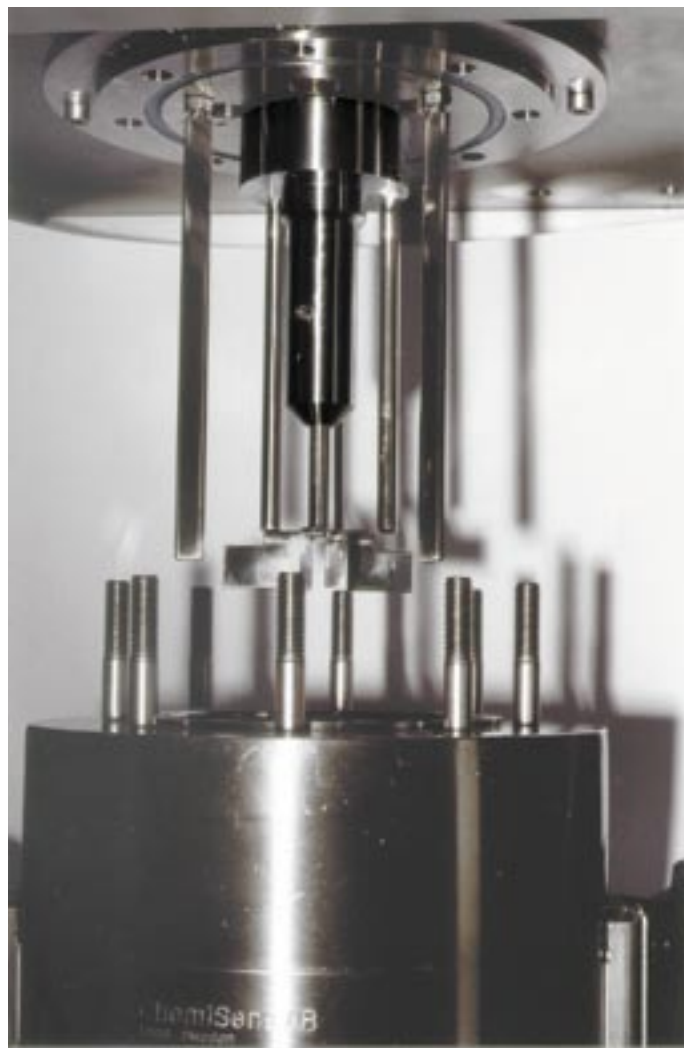
Internal torque transducer with turbine stirrer mounted. Three baffles are also installed in the reactor lid.
