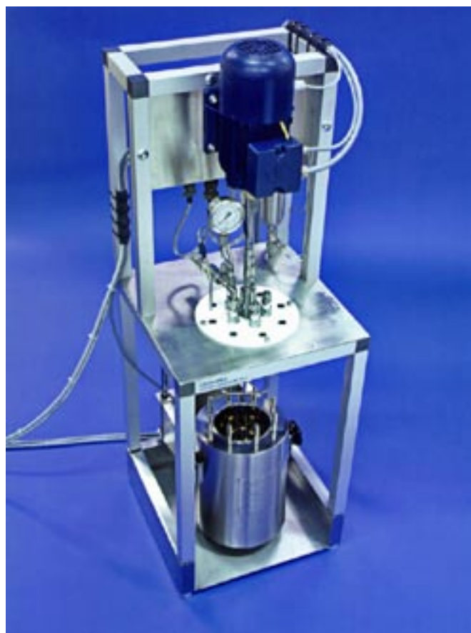
The bench unit with the 25 bars reactor.
