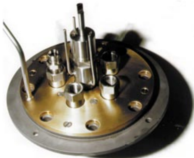
Tantalum plated lid - 25 bars reactor - with the lid heating plate installed.
