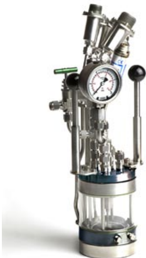
Tantalum reactor for pressures up to 20 bars.
