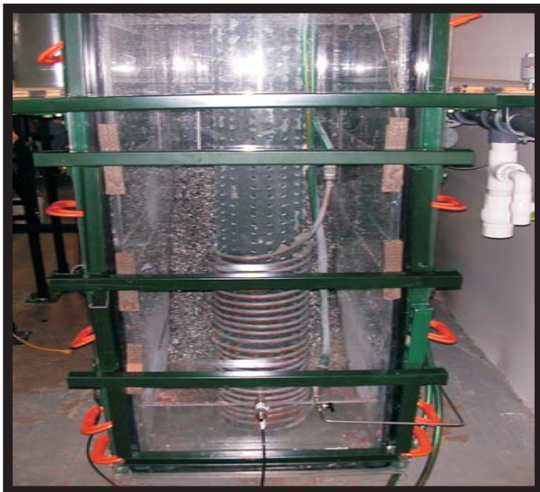
Discharge side view, which shows the sparger and cooling coil. The cooling coil is used for extended duration test to maintain a constant water temperature.
